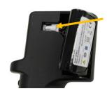
Push down on connector latch and pull battery loose from the board.
