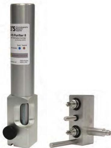
A high-capacity gas purifying system that removes moisture and hydrocarbons, (greater than C4) from air, inert gases and hydrogen. It contains a high-sensitivity moisture indicator. When the cartridge is depleted the moisture indicator changes from BLUE to BROWN. The AFS Purifier II can be expected to supply multiple GC installations for an extended period of time depending on the laboratory environment.
